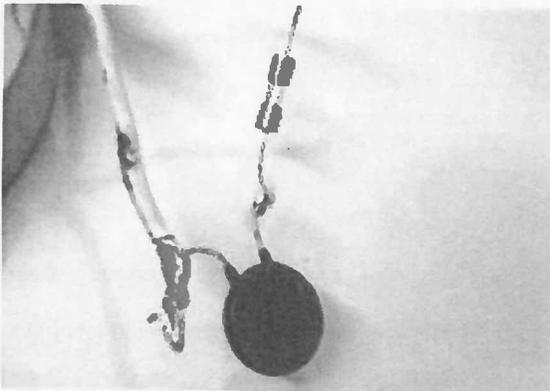
Figure 15. A 3-amp, slow-blow, 350-volt line fuse and 510-volt MOV after one 2.5-kV surge: opened fuse, no damage to MOV.
