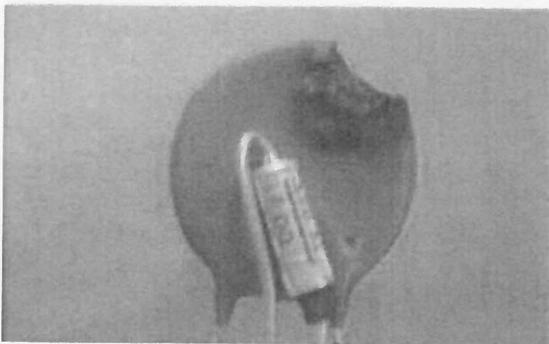
Figure 10. A ceased MOV failure caused by interruption of the conduction current by an external TCO (adapted from Littelfuse, Inc.).
