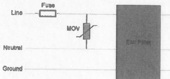
Figure 2. Basic AC power input protection circuit for end-use equipment.
